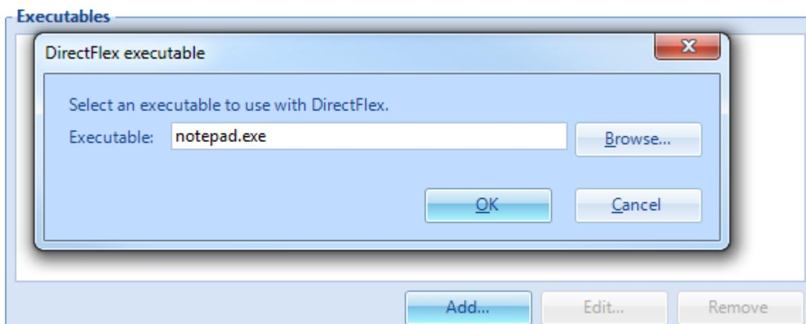
You can either specify the complete path, or just the executable name (which, as is the case in the example above, can be convenient if there are multiple copies in different locations – as an alternative you can of course also specify the full path of each copy).
