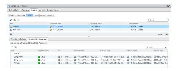
This next screenshot is taken from the VMDK – Hard disk 1. It implements both the stripe width (RAID 0) and the failures to tolerate (RAID 1) requirements. There are a total of 5 components making up this object; two components are striped, and then mirrored to another two-way stripe. Finally, the object also contains a witness component for quorum decisions.
