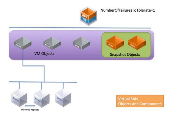
Each of these objects is comprised of a set of components, determined by capabilities placed in the VM Storage Policy. For example, if *NumberOfFailuresToTolerate=1* is set in the VM Storage Policy, then the VMDK object would be mirrored/replicated, with each replica being comprised of at least one component. If *NumberOfDiskStripesPerObject* is greater than one in the VM Storage Policy, then the object is striped
