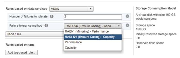
For FTT=1 the storage overhead will be 1.33X rather than 2X. In this case a 20GB VMDK would use on 27GB instead of the 40GB traditionally used by RAID-1.
